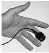
Figure 20. Attachment using an elastic band.
